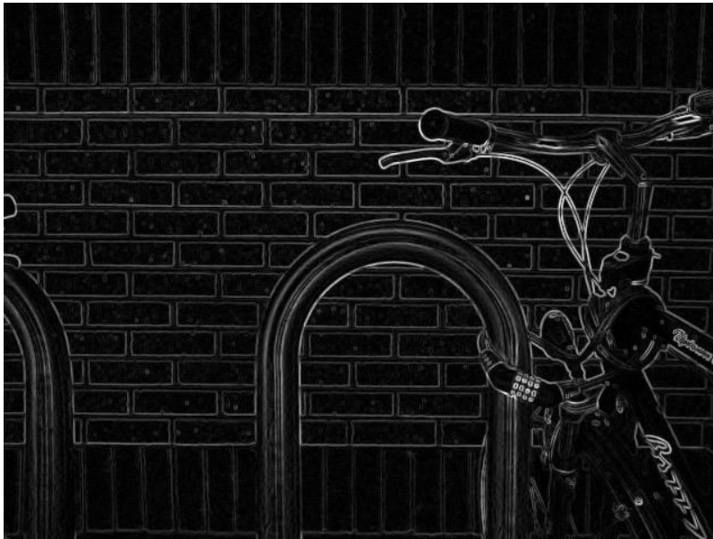
Figure 6. Gradient magnitude from Prewitt operator [26]
