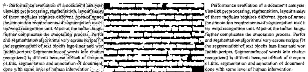
Figure 21. The final result (right) obtained after combining the binary image (left) with the dilated gradient map (center).
